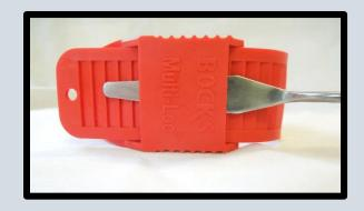
Insert a thin flat object between the top of the buckle and the serrated surface of the band in the direction the strap enters the buckle. This will release the serrations and the band will come loose, ready for possible reuse.
